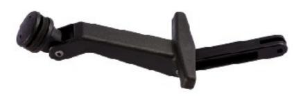
This easy to operate window hold-open is designed to fit comfortably in the hand for top and side hinged venting windows for on and off-highway vehicles. It features an over center design that orientates the window at fully closed and fully open positions and an optional quick release pin in bright red nylon or steel.
